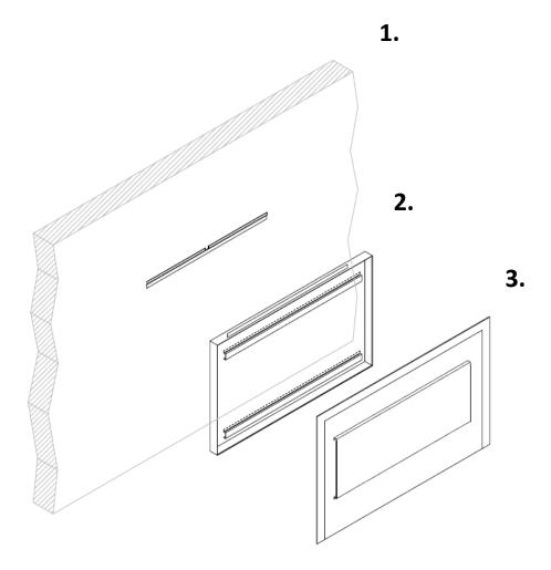
Step 1. Level and attach cleat to wall.
