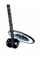
FEATURES: This convex inspection mirror provides a wide angle view to scan large areas quickly. The black powder coated handle is adjustable from 30" to 50". The mirror rests on 4" wheels and is available in glass or acrylic. It is constructed with a holding bracket for a standard "D" flashlight, (flashlight not included).
