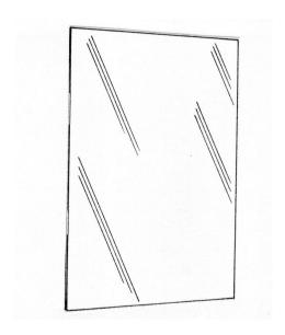
MIRROR: 1/4" inch thick, electro-copper plated, consisting of silver coating, copper coating, baked on backing paint, equal to and conforms to the applicable portions of Federal Specification DD-M-00411 and shall be Type1/Class1/Quality Q2 and complies with ASTM C1036-91.
