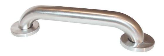
MATERIALS: Stainless steel Type 304, 18 gauge tubing with No.4 satin finish. Mounting back plate is 12 gauge, Type 304 stainless steel, 3" (76 mm) in diameter and heliarc welded to bar. Snap flange cover escutcheon is 22 gauge, Type 304 stainless steel polished with No.4 satin finish. Escutcheon cover is for concealing screws, esthetics only. All flanges and center post are heliarc welded to tubing forming an integral part of the bar. The grab bar is available in 1", 1-1/4" and 1-1/2" diameter.
