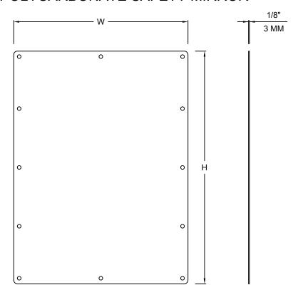
MIRROR: NUMBER 1 QUALITY POLYCARBONATE, .125 INCH THICKNESS. MINIMUM TENSILE STRENGTH WILL BE 9,000 PSI (ASTM D-638), COMPRESSIVE STRENGTH: 12,500 PSI (ASTM D-695), FLASH IGNITION TEMPERATURE: MUST EXCEED 870 DEG F, AND IZOD IMPACT STRENGTH-MOLDED NOTCH OF 12 FT-LB/IN NOTCH (ASTM D-256).
