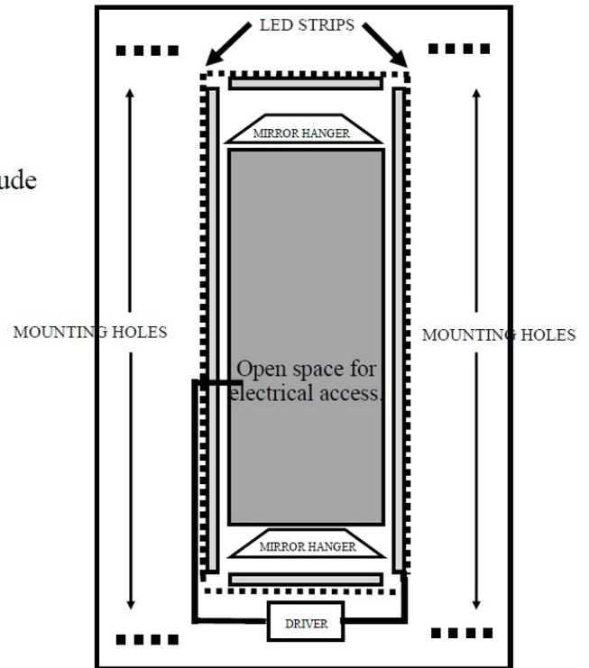
◀ **SPECIFICATIONS:** 5mm polished silver mirror & white powder coated steel base. Lamp 5050 SMD LED, 6000K. With UL certified defogger pad, with ON-OFF Switch. AC110-120V, 50/60Hz. Built in electronic LED driver (Must be installed by licensed electrician). Meek Mirrors wall hanger and theft proof system.
