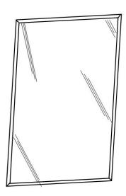
MIRROR: Electro-copper plated, consisting of silver coating, copper coating, baked on backing paint, equal to and conforms to the applicable portions of Federal Specification DD-M-00411 and shall be Type1/Class1/Quality Q2 and complies with ASTM C1036-91.
