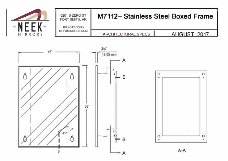
MIRROR: 1/2 thick, electro-copper plated, consisting of silver coating, copper coating, baked on backing paint, equal to and conforms to the applicable portions of Federal Specification DD-M-004 11 and shall be Type 1/Class 1/Quality Q2 & complies with ASTM C1036-91.
