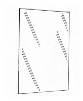
MIRROR: 1/4" inch thick, electro-copper plated, consisting of silver coating, copper coating, baked on backing paint, equal to and conforms to the applicable portions of Federal Specification DD-M-00411 and shall be Type1/Class1/Quality Q2 and complies with ASTM C1036-91.
