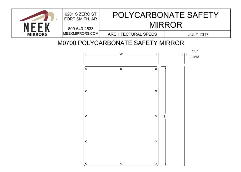
MIRROR: NUMBER 1 QUALITY POLYCARBONATE, .125 INCH THICKNESS. MINIMUM TENSILE STRENGTH WILL BE 9,000 PSI (ASTM D-638), COMPRESSIVE STRENGTH: 12,500 PSI (ASTM D-695), FLASH IGNITION TEMPERATURE: MUST EXCEED 870 DEG F, AND IZOD IMPACT STRENGTH-MOLDED NOTCH OF 12 FT-LB/IN NOTCH (ASTM D-256).
